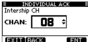
④ The Individual ACK confirmation screen is displayed. Push [CALL] to transmit an acknowledgement call.
