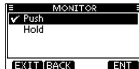
**Push** : The monitor function is activated by holding down [VOL/SQL] for 1 second. The squelch opens while holding down the key.
