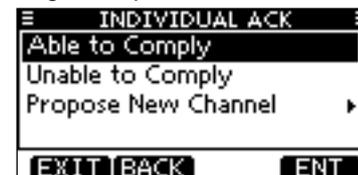
When “INDIVIDUAL ACK” is set to “Auto ACK (Unable),” the transceiver automatically replies to the Call. In that case, both the TX and RX calls are stored in the Transmitted and Received Call Logs.
