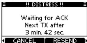
⑥ After receiving an acknowledgment call, push [ALARM OFF] then reply using the microphone.
