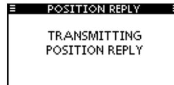
When “POSITION ACK” is set to “Auto TX,” the transceiver automatically replies to the Call. In that case, both the TX and RX calls are stored in the Transmitted and Received Call Logs.
