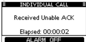
Push [ALARM OFF] to stop the beeps. Then push [EXIT] to return to the operating channel (before you entered the MENU screen).
