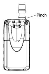
To make your scanner easier to carry when you are on the go, use the supplied belt clip. Slide the belt clip into the hanger piece on the back of the scanner. To remove, slide up the belt clip pulling the pinch at the middle of the belt clip.
