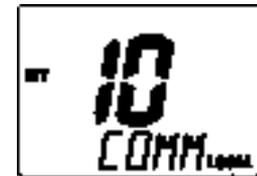
Appears when the RF attenuator function is in use
